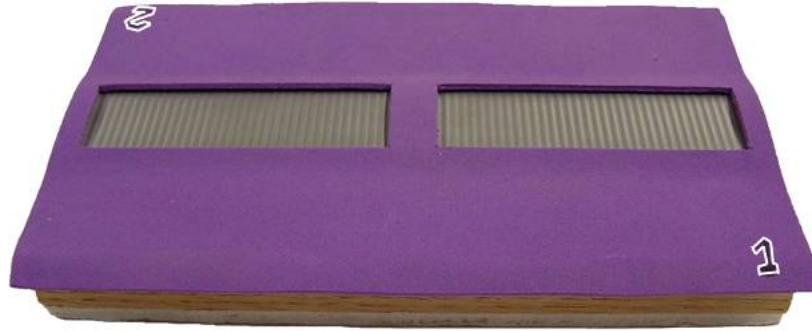
Fig. 3.9.: The test apparatus for holding two stainless steel blocks with surface gratings. The numbers “1” and “2” were used by the experimenter to determine which grating should be presented to the left of the participant on each trial. The apparatus was always obscured by a curtain from the participant’s view.
